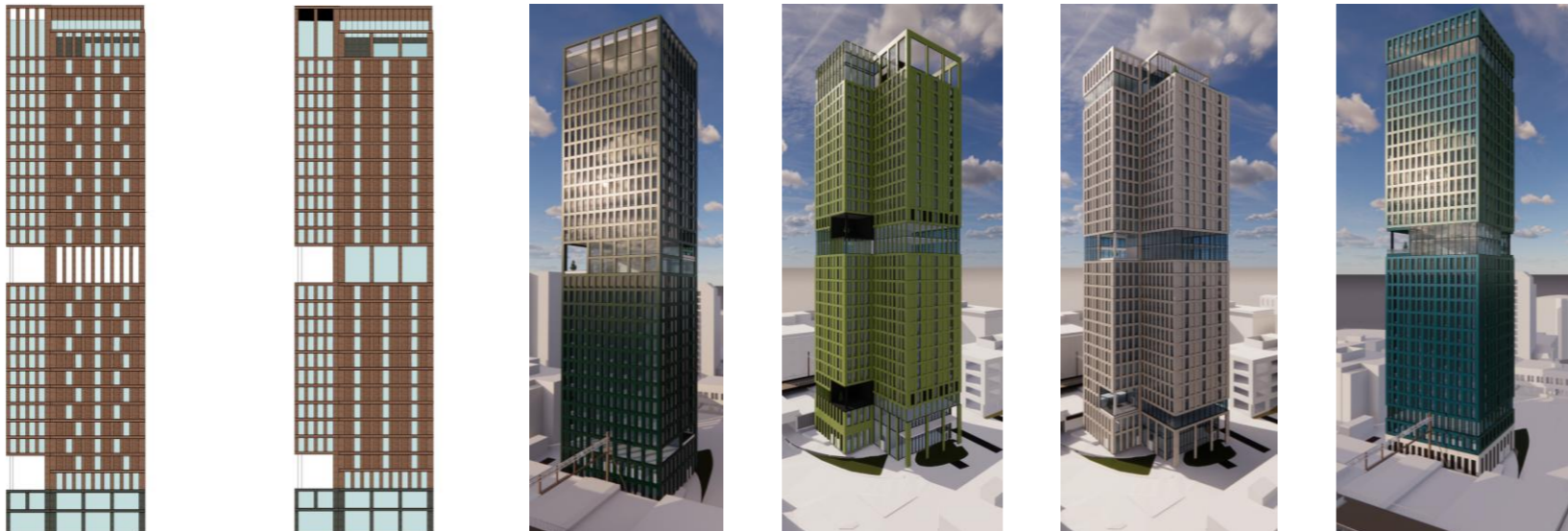
Exploration of colour treatments, fenestration patterns and differentiation of the top, middle and base of the building and façade articulation.
